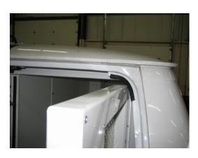
Note: It is recommended to put edge molding on the OEM door opening on the passenger side to avoid damaging the Kwik kit door.
